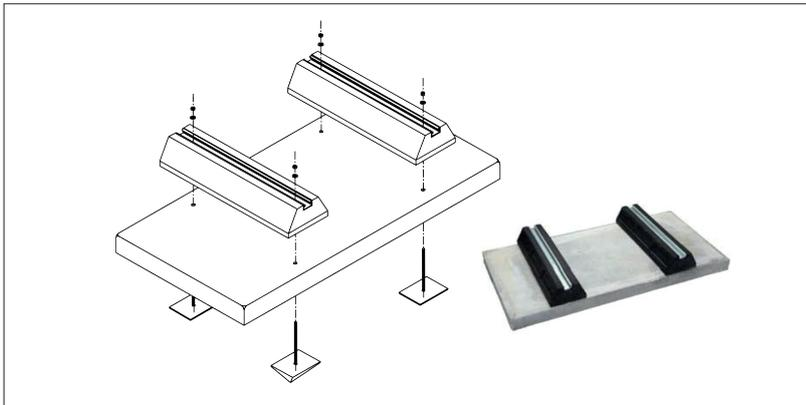
A low cost innovative solution for floor mounting air conditioning units and ASHP. The FLEXI Lite Slab and Foot kit avoids the high cost and time consuming need to construct a concrete base and comes complete with FLEXI rubber mounting feet. It can be delivered to site with minimum preparation and can be assembled in minutes. It also suits most brands of domestic air source heat pumps and air conditioning units.
